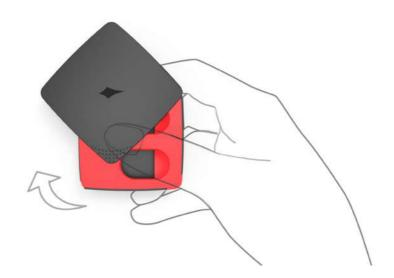
Open the dock by using the grip area to slide the cover clockwise.
